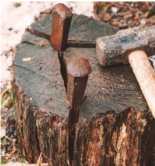
Figure 9: Worn splitting wedges, note the burrs which require removal.
