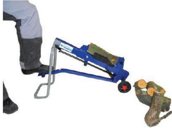
Figure 12: Example of a foot-operated splitter
