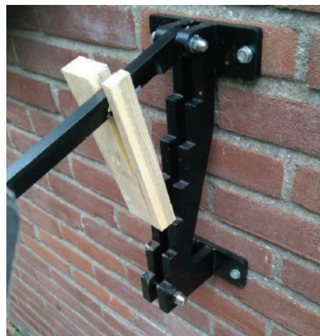
Figure 16: Wall-mounted kindling splitter
