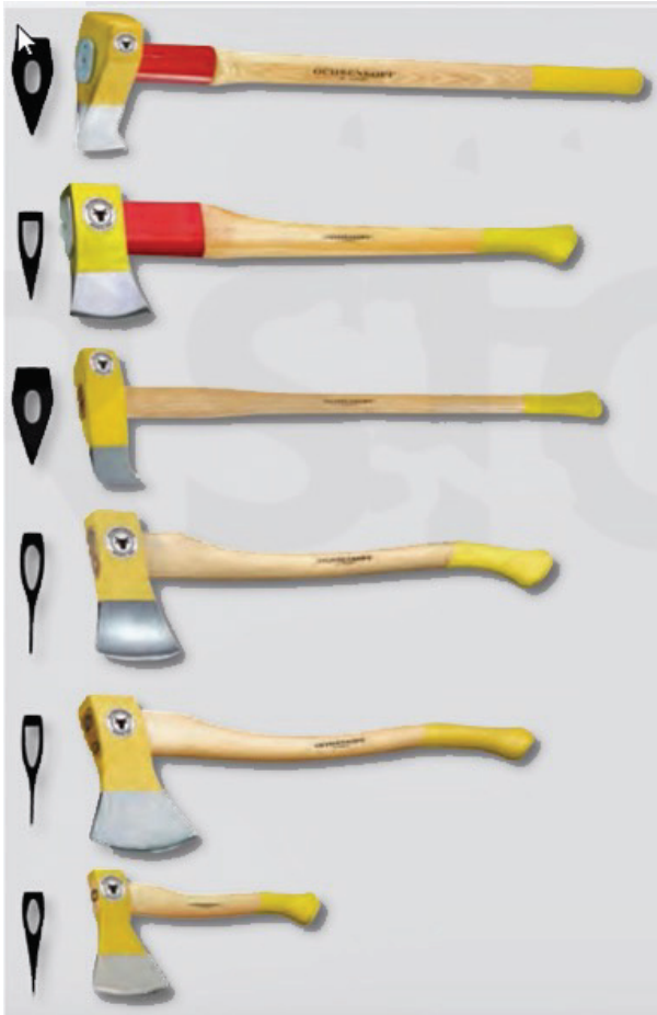
Figure 5: Types of axe, the top three are used for splitting, the next two are for delimiting and the bottom one is a simple chopping axe. Note the profiles to the left of each axe.
