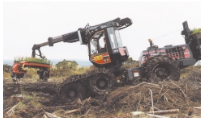
Figure 7: Machines used for planting container stock.
