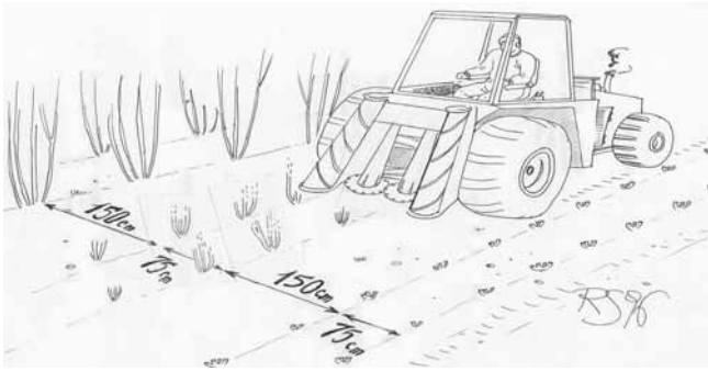
Figure 1: Recommended planting configuration of short rotation coppice willow to facilitate harvesting.
