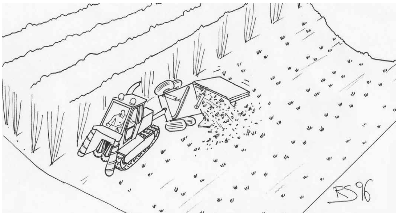
Figure 10: Avoid planting willow crops along the slope as machines may become unstable during harvesting.
