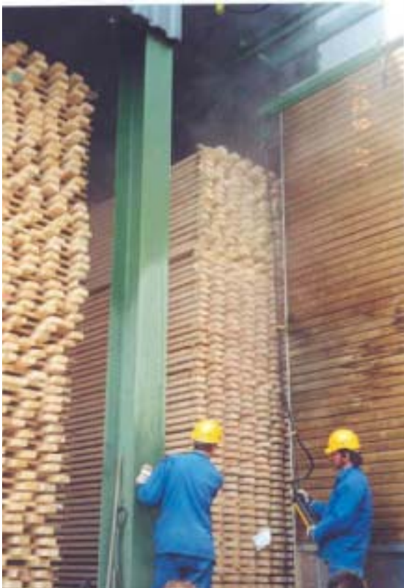
Figure 5: A load of timber being extracted from a kiln drier. The control of moisture is a vital component of the correct use of timber products.
