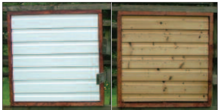
Figure 9: Painted and unpainted heat treated Sitka spruce panels under outdoor exposure test at BRE.
