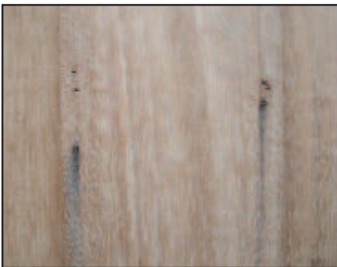
Figure 4. Staining in iroko from mild steel nails.
