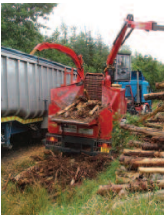
Figure 11: Starchl chipper blowing chips into truck.
