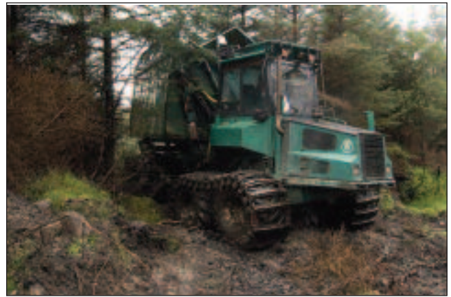
Figure 10: Silvatec chip forwarder leaving the extraction rack with a load of chips.
