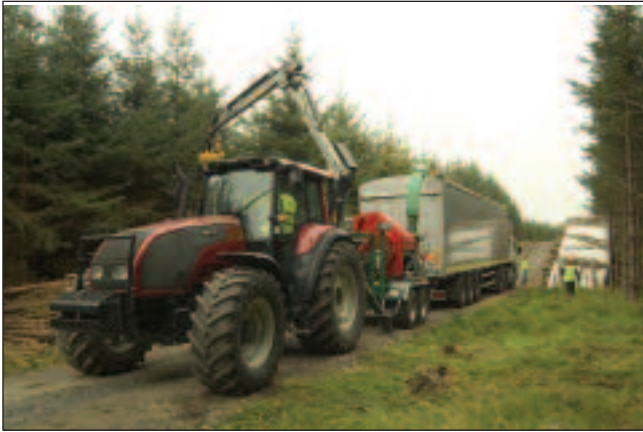
Figure 7: MusMax tractor-powered chipper blowing chips into a walking floor truck.
