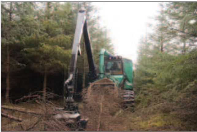
Figure 9: Silvatec terrain chipper on band tracks in a line thinning.
