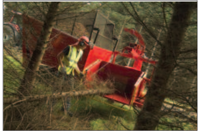
Figure 8: TP230 winching a tree into the chipper.
