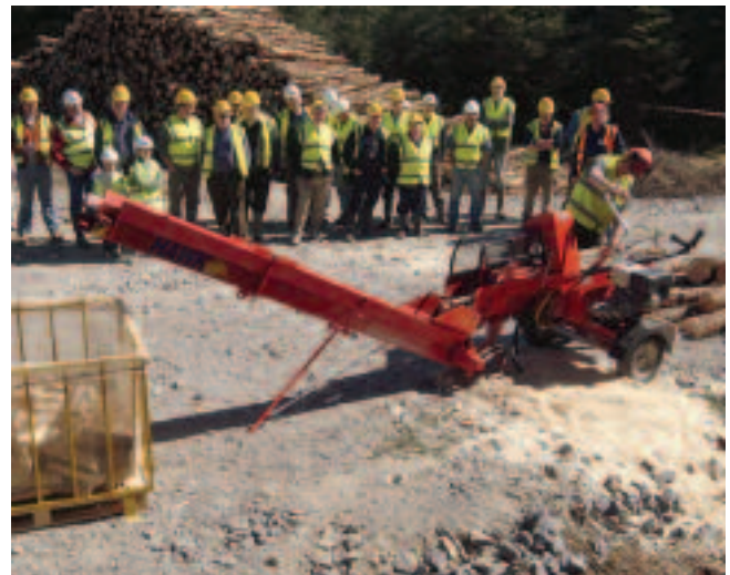
Firewood processing with the Hawk firewood processor during one of the harvesting demonstrations.
