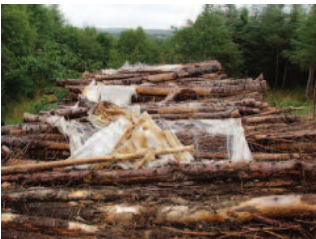
Disintegrated paper cover after 15 months storage.
