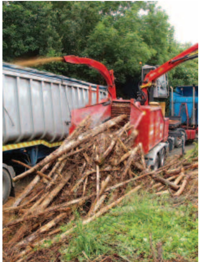
Breakage during chipping due to partial decomposition of the wood following prolonged storage.
