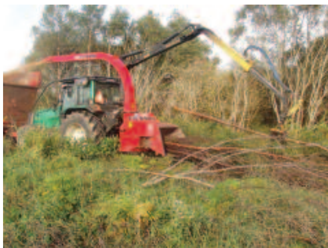
Tractor-mounted chipper working on clearfell of naturally-regenerated birch.
