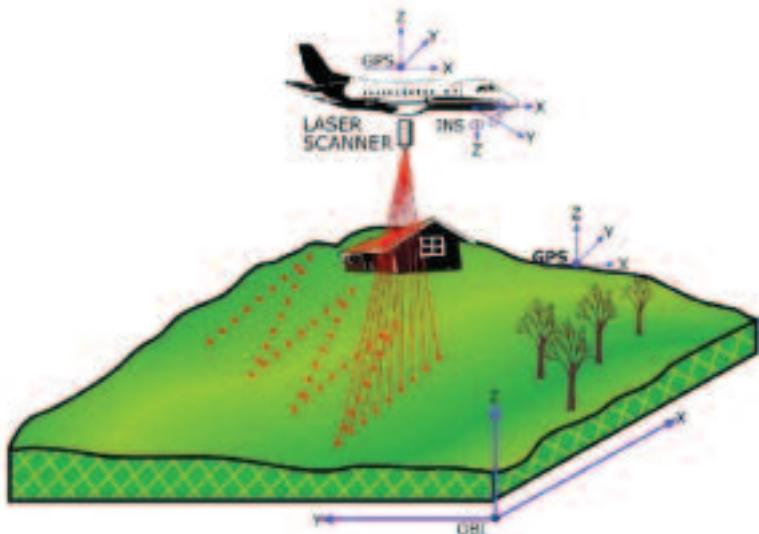
Figure 1: Aerial LiDAR scanning, using differential GPS for positioning and orientation (after Renslow et al. 2000).
