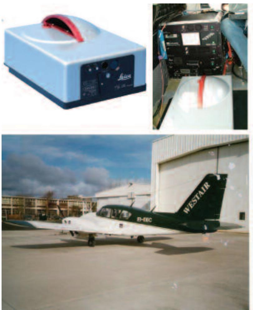
Figure 3: Leica aerial laser scanner (top), mounted on a computer and the aircraft used.
