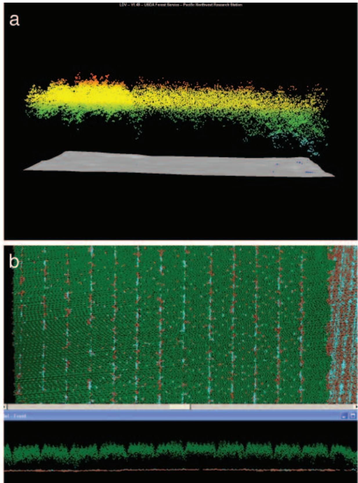
Figure 4: First returns displayed over the surface model to create a canopy surface model (a) and plan and elevation view of stand showing thinning racks and ground surface level and tree height (b).
