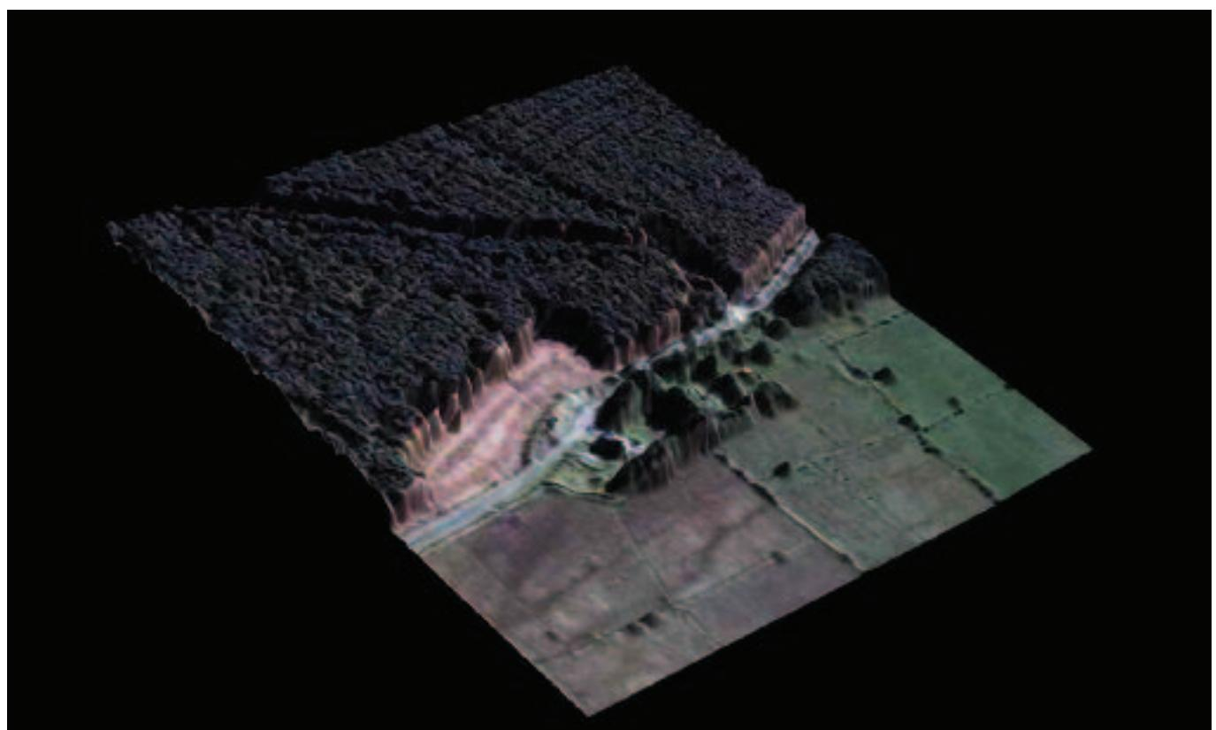
Figure 6: Exaggerated 3D canopy surface layer derived from LiDAR enhanced with digital orthophotography (Quickbird), showing stand structure, bell mouth entrance and main extraction racks.
