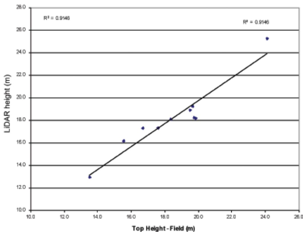
Figure 7: The relationship between field-based top height and LiDAR-derived height.
