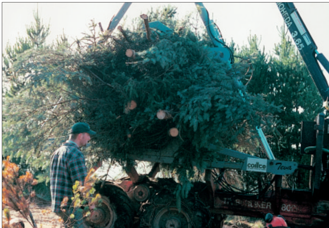
Figure 17: The bundler compacting some fresh green spruce (note the base of the bundler is well above the tyres).
