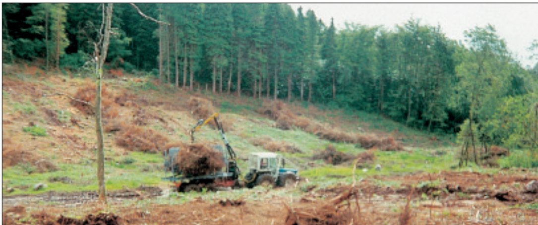
Figure 11: The prototype Limerick bundler working with windrowed residues at Murroe, Co Limerick.
