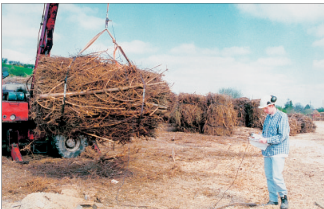
Figure 13: Bundle being weighed using customised loadcell.
