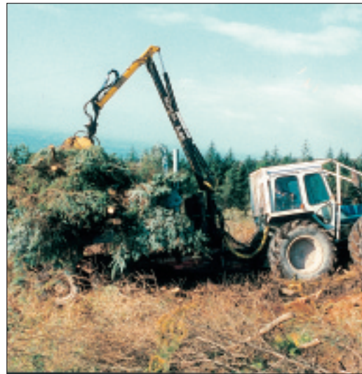
Figure 18: Boom of crane was too close to rams of bundler.
