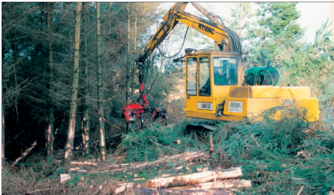
Figure 1: Hymac excavator fitted with a harvesting head placing wood lengths alongside residues which form a brash mat under the tracked vehicle.
