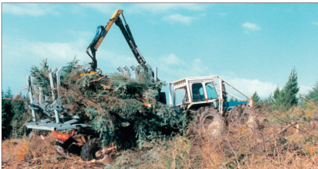
Figure 12: The bundler working at Buffanoka loading (fresh) green residues from a brash mat.
