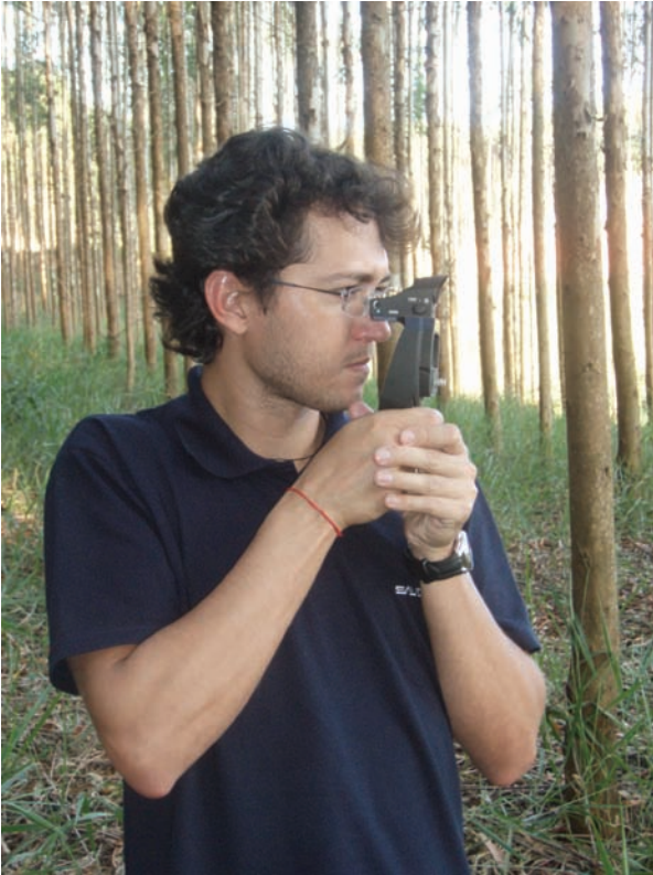
Figure 1: The Masser RC3H in use, a basal area calculator for productive inventory and planning work. This forms part of the measurement equipment database developed during the TREEMODEL project.
