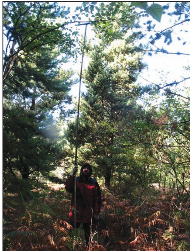
A peat auger at 6 m extension used to collect samples from varying depths through the soil profile.
