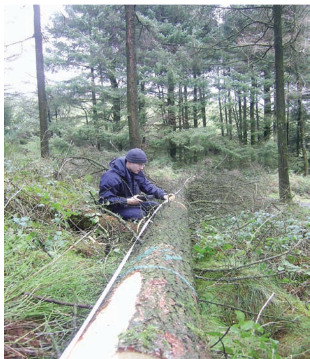
Figure 1: Sectional measurement of a Japanese larch sample tree, Virginia Forest, Co Cavan.
