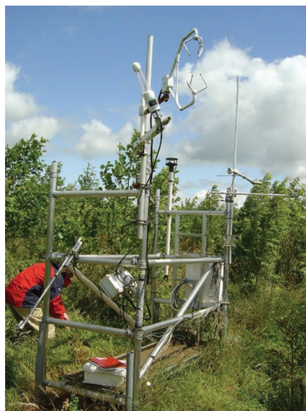
Figure 4: The eddy covariance flux tower.
