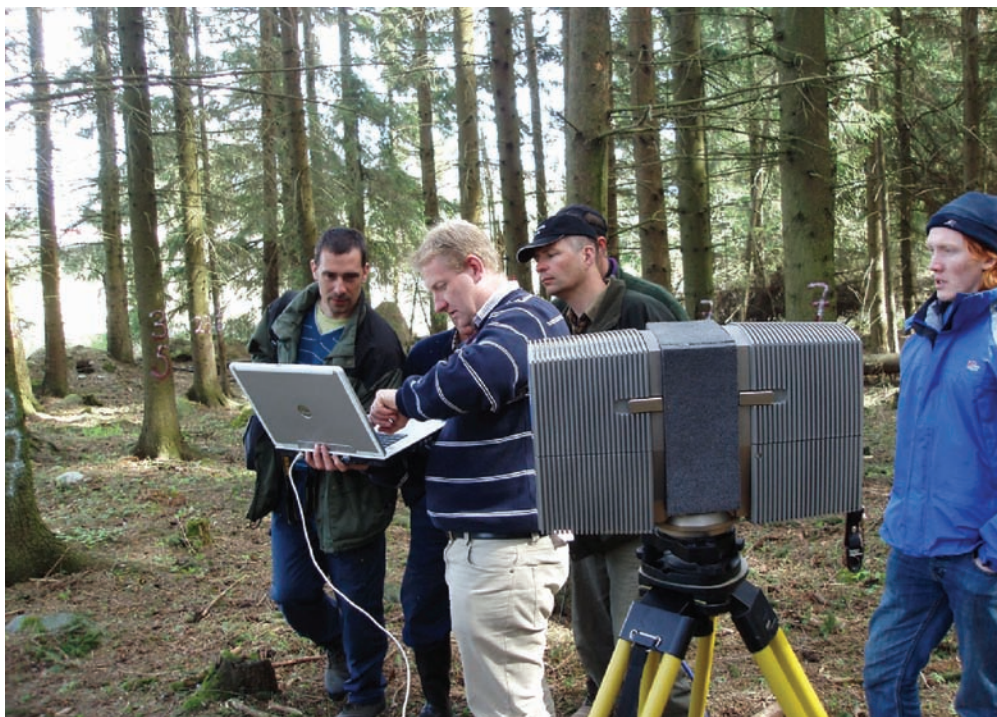
Figure 1: Data collected from the scanning device (foreground) is uploaded to a computer. The resulting point cloud data is processed to arrive at stem diameter distributions.
