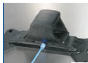
Figure 1: Jost fifth wheel load cell.
