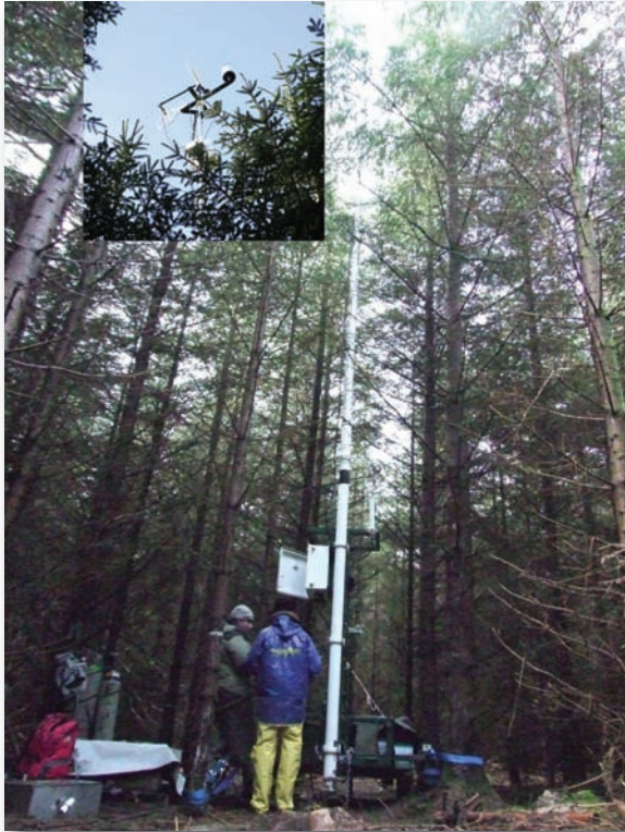
Figure 1: The roving eddy covariance system designed to move between selected sites to assess net C balance (NEP) of stands following afforestation, thinning and harvest. Insert shows the instrumentation attached to the top of the mobile tower.
