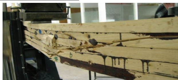
▲ Flexure testing of Irish-grown Sitka spruce glulam.
