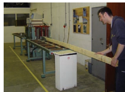
▶ Mechanical grading of laminations.
