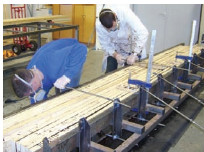
◀ Manufacture of glue-laminated beams.
