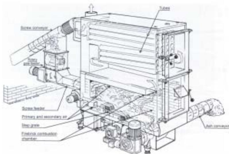
**Figure 6: Automatic Wood Chip-fired Heating System**
