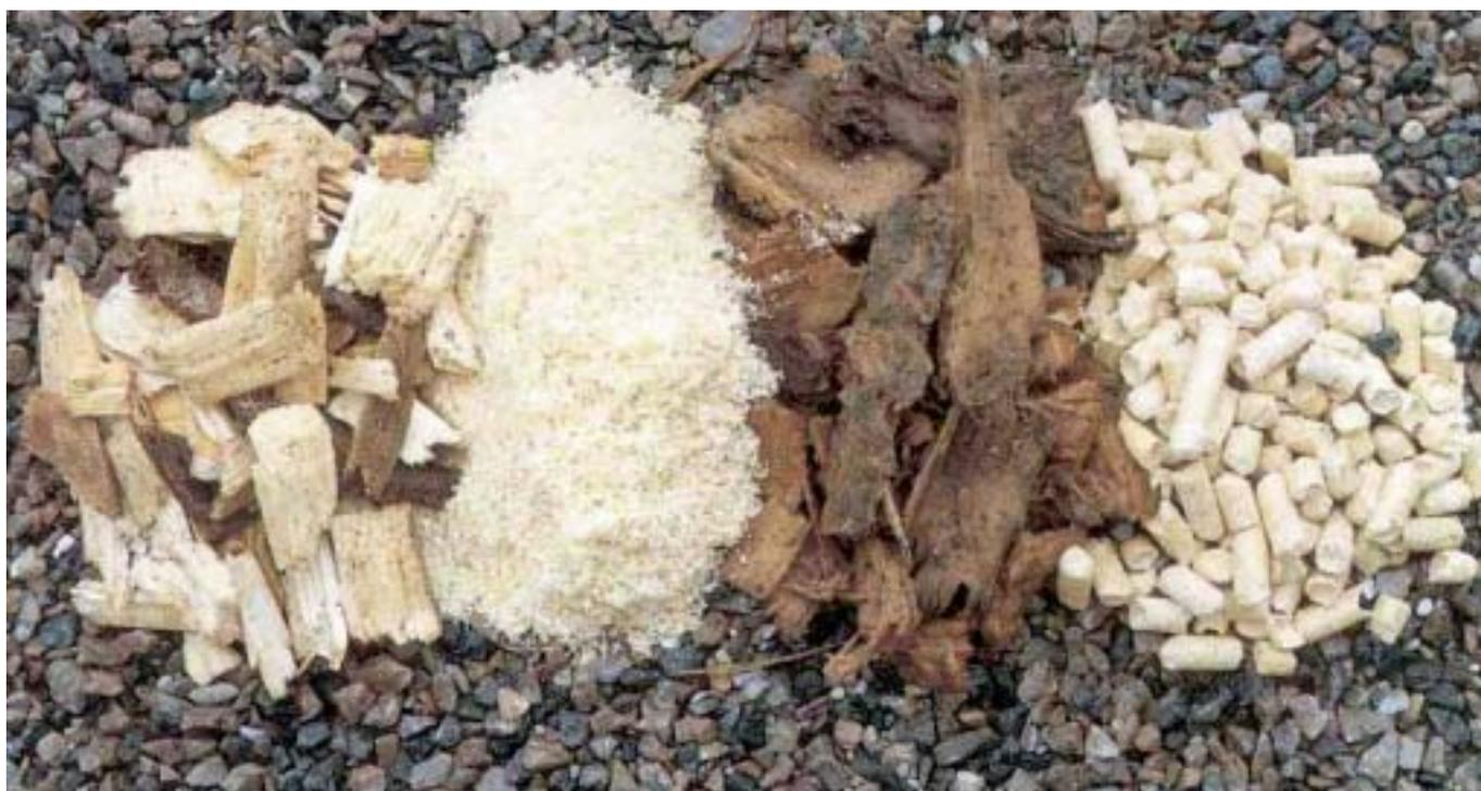
**Figure 5: Forms of Wood Fuel Forest wood chips, sawdust, bark, wood pellets**
