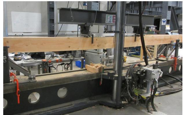
Figure 2: Destructive bending test on Douglas fir specimen at NUIG.
