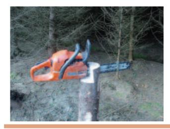
Step 6: Insert the chainsaw with the blade in the opening and with the machine resting on the step (if the spikes on the chainsaw have been maintained, ram them into the upright) and fix the machine in place with the nut tightening key.
