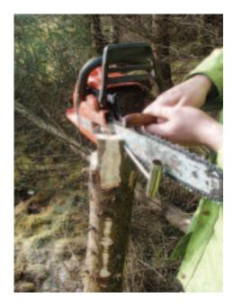
Now the chainsaw can be sharpened while the operator is standing up.
