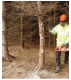
Step 4: Cut a step 15 cm deep about 4-5 cm from the edge of the trunk.
