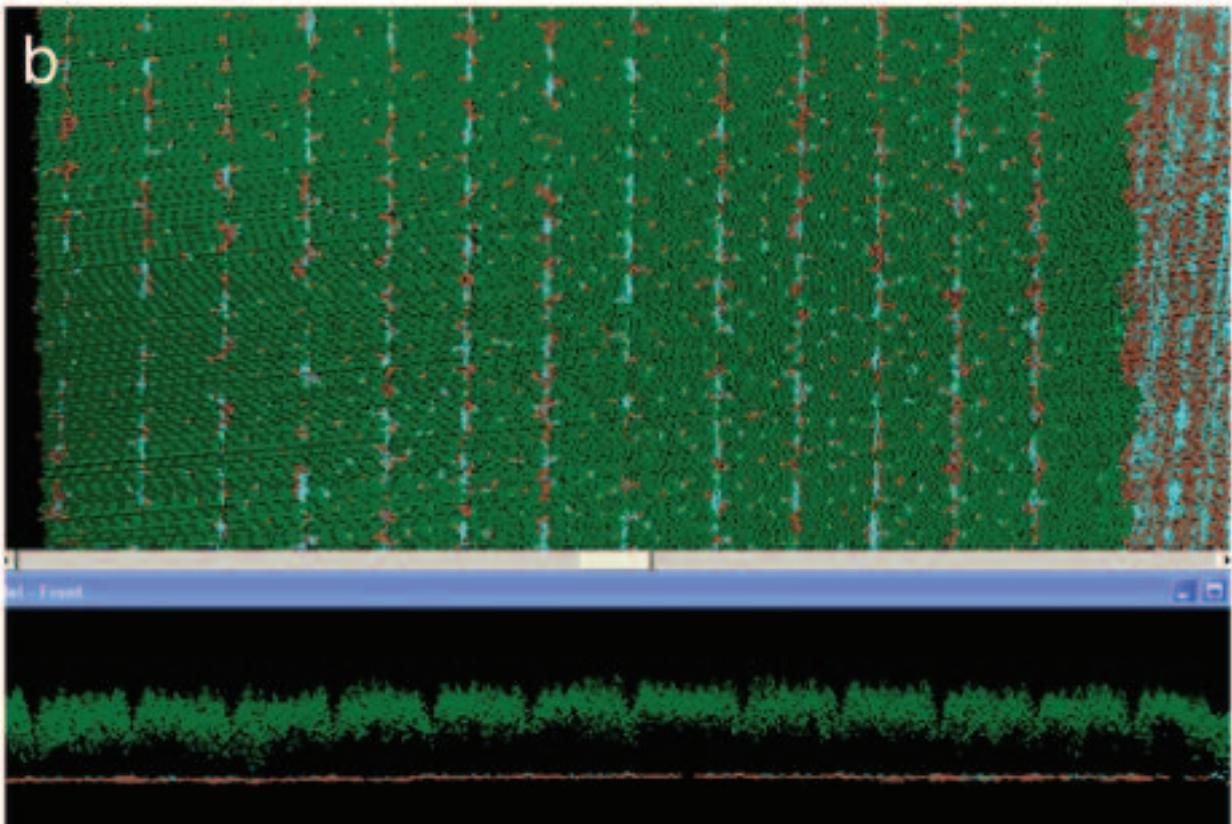
Figure 4: First returns displayed over the surface model to create a canopy surface model (a) and plan and elevation view of stand showing thinning racks and ground surface level and tree height (b).
