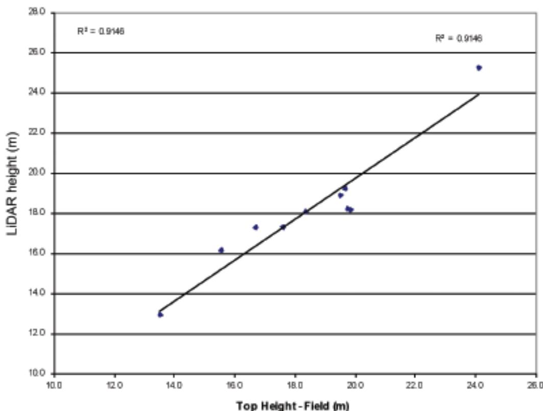
Figure 7: The relationship between field-based top height and LiDAR-derived height.
