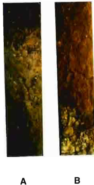
Photograph 1. A comparison of an impermeable soil (A) and a free-draining soil (B). In A, a thin (150mm) dark organic topsoil overlies a dark grey cohesive, plastic and impermeable clay. In B, a brown brittle topsoil of about 600 mm overlies a light grey brittle loamy subsoil.
