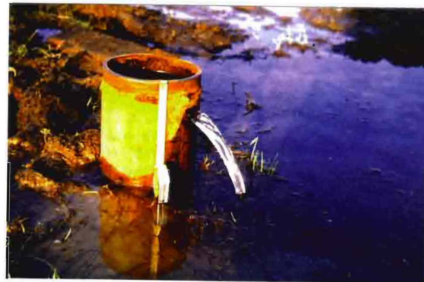
Photograph 4. The artesian (central) well of Transect 1 showing a free discharge of 4m 3 /hr at ground surface
