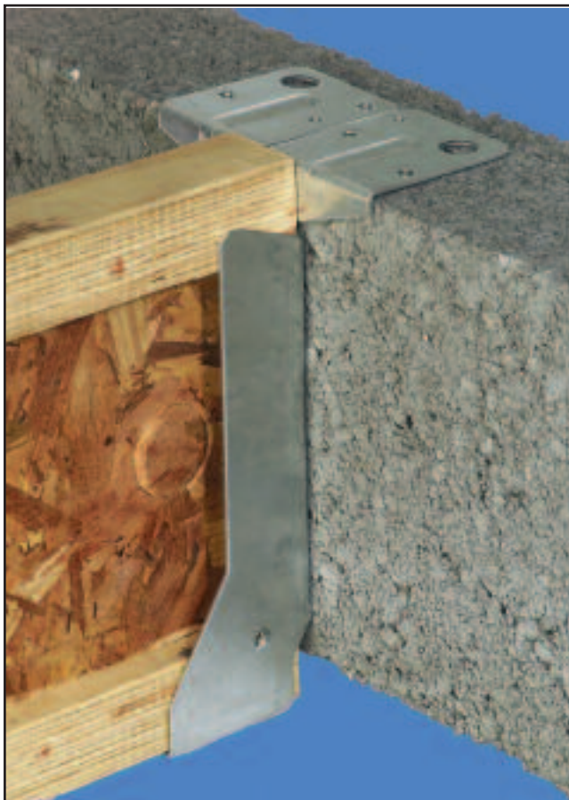
▲ I-joist attached to masonry wall with a specialised hanger. Many EWPs are supplied as a package that includes fixings and other ancillary products.
