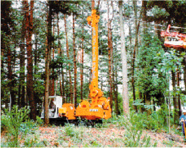
Figure 22: Iwafuji TY-U3 tower yarder mounted on a crawler base using self propelled carriage
