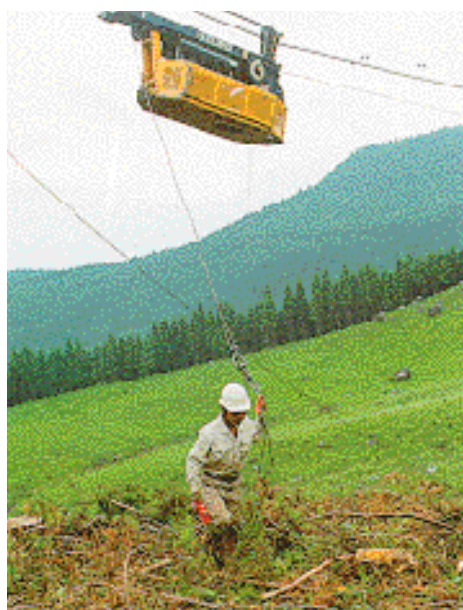
Figure 23: Sky-carry remote controlled self-propelled carriage
