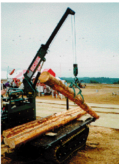
Figure 18: A typical small forwarder of the side loading type (top) and a small forwarder with trailer (bottom)
