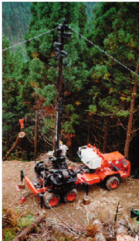
Figure 21: Oikawa Motors RME 200 tower yarder with all terrain base machine
