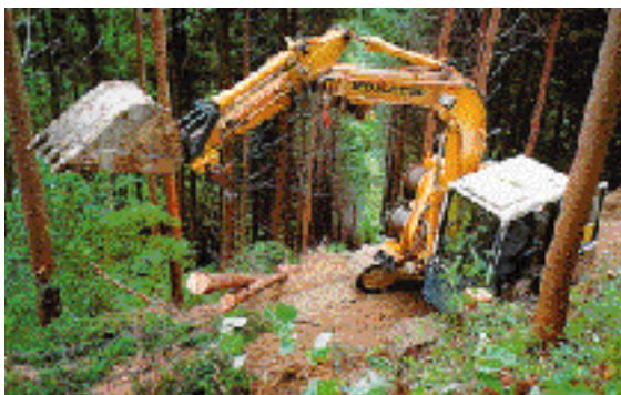
Figure 23: HC 20 model swing yarder from the Komatsu company
