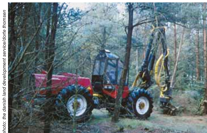
Figure 7: The feller-buncher, which is a narrow off-road machine with a crane mounted saw felling head, fells the thinning trees and arranges them in rows, so that the chipper can subsequently chip them after drying for a couple of summer months.
