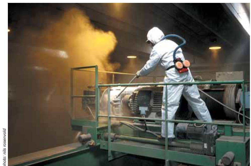
Figure 24: Worker at Måbjergværket wearing P3 filter respirator for toxic particles during the cleaning of machinery.
