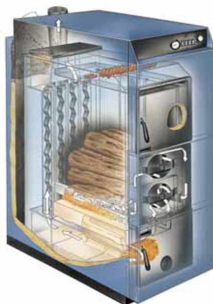
Figure 29: "X-ray" of manually fired boiler. The magazine is almost half full of fuelwood, and the combustion is in the form of downdraft combustion, i.e., the burning gases pass down through a lined chamber, where the combustion is completed. The combustion air is introduced through inlets in the gate and is pre-heated. The flue gases move backwards and pass the tubes (the convection unit). The tubes are equipped with spirals so as to increase the amount of heat being given off to the boiler water. An exhaust fan at the back of the boiler ensures a correct negative pressure in the combustion chamber.
